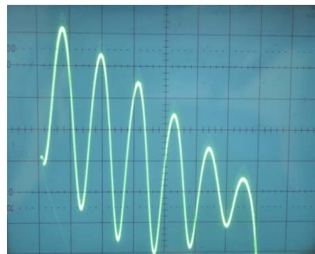
Fig. 4 Oscilloscope display of Frank-Hertz Experiment
